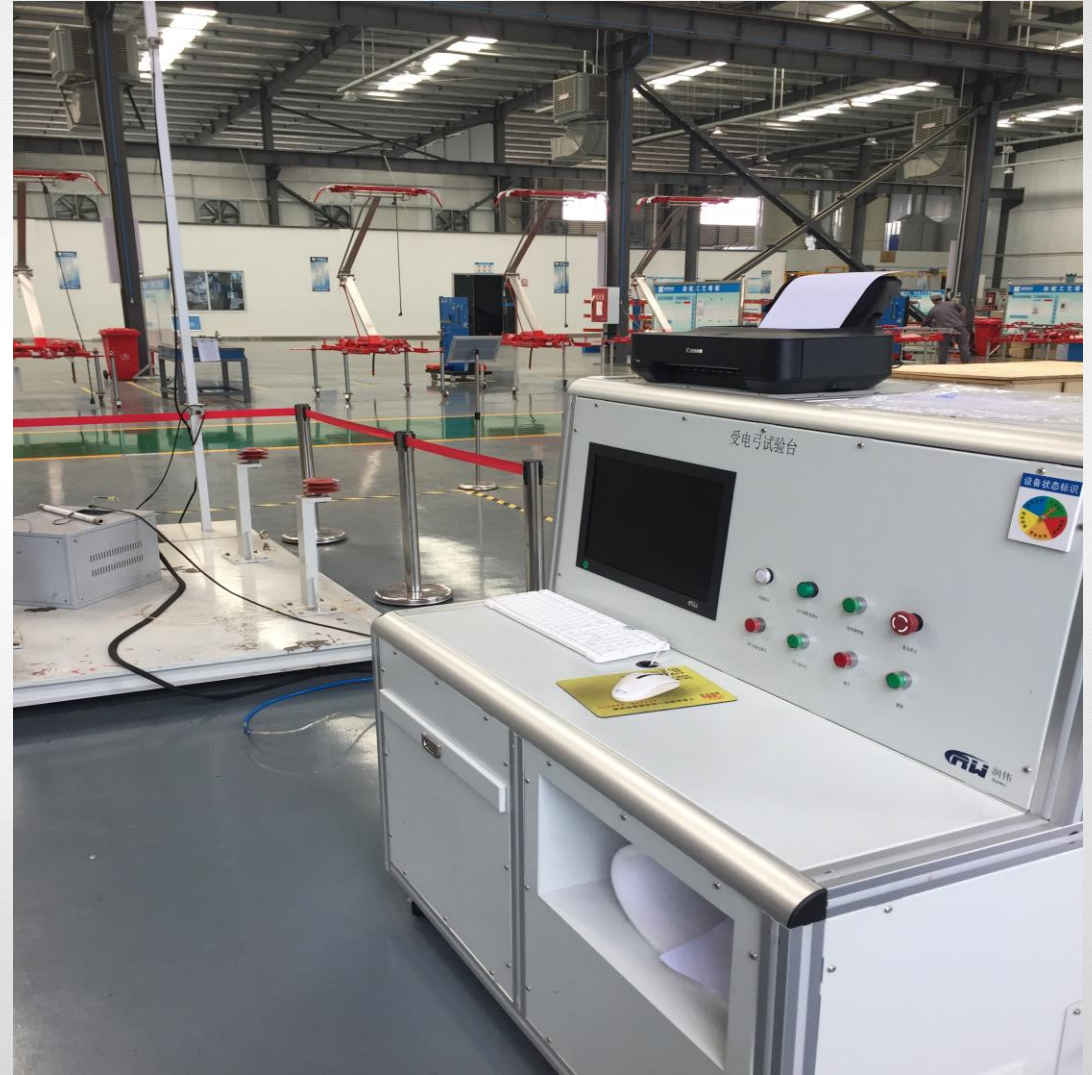
Pantograph test machine
